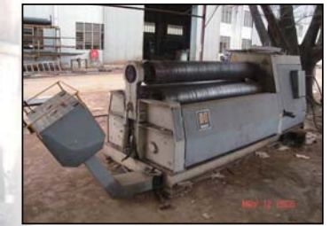
HACO 3HBR220 Rolling Machine Capacity : MS Plate Thickness 1mm ~ 12mm
