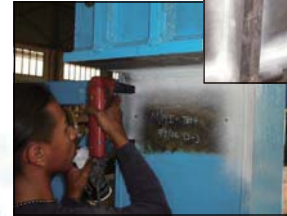
MPI Test on Pier Bracket & Internal Strut.
