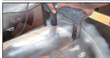
Magnetic Particle Inspection (MPI) Test In Progress on Fillet Weld.
