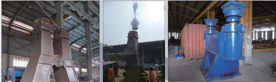
Front Support Sub-Frame Trial Assembly.
