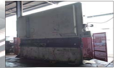
500 tons Press Brake Capacity : MS Plate Thickness 1mm ~ 12mm @ 3000mm LG
