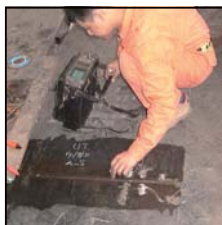
UT Test In Progress on Butt Weld.
