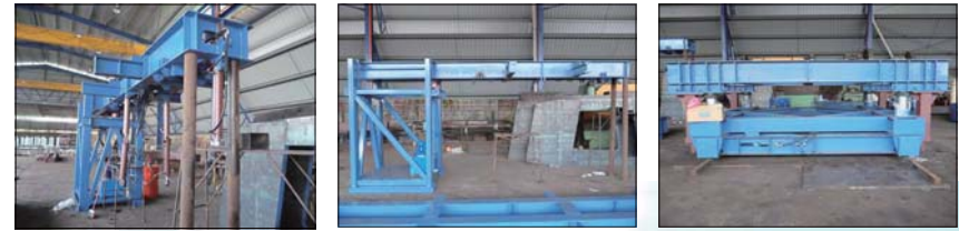
Inner core arm & hydraulic operation trial test at factory.
