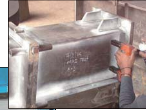
MPI Test on Pier Bracket & Internal Strut.
