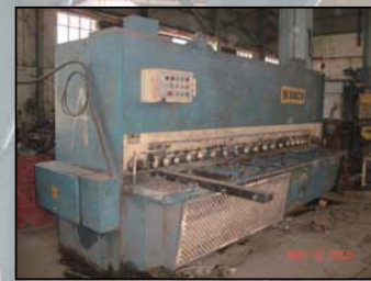
HACO HSLX 3013 Shearing Machine Capacity : MS Plate Thickness 4.5mm ~ 10mm
