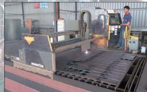
Komatsu Plasma CNC Profiling Cutting machine Size 2000mm X 6000mm Capacity : Mild Steel 50mm thk / Stainless Steel 30mm thk
