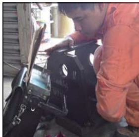
UT Test In Progress on Butt Weld.
