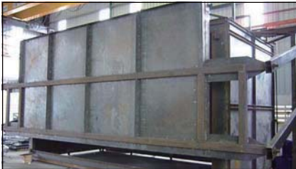
Heating Tank with swing door
