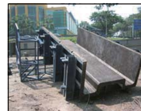
Column Steel Mould
