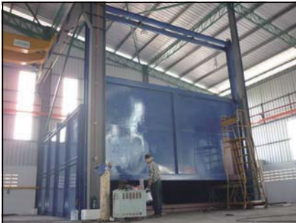
Heating Tank with slide door
