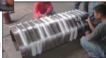
UT Test In Progress on Butt Weld.
