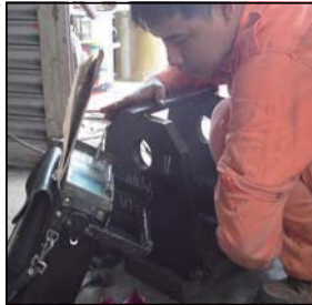
UT Test In Progress on Butt Weld.
