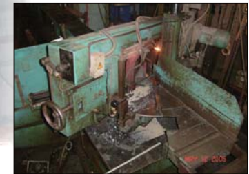
360MM KALTENBACH CIRCULAR BENDSAW ( DEGREE TYPE )
