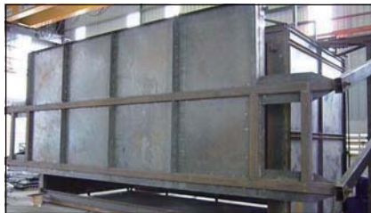
Heating Tank with swing door
