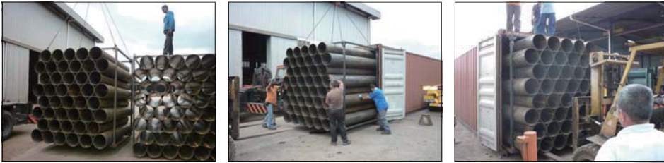
Casing pipe for site piling works.
