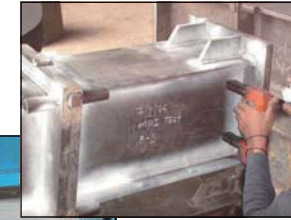
MPI Test on Pier Bracket & Internal Strut.
