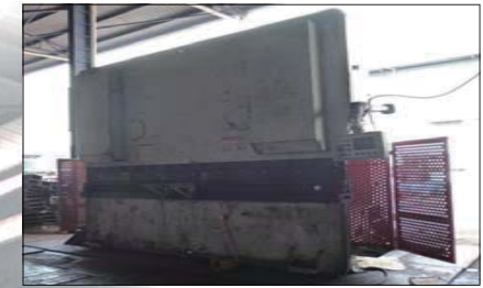
500 tons Press Brake Capacity : MS Plate Thickness 1mm ~ 12mm @ 3000mm LG
