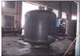
In house fabrication of Blow Pod for Dense Phase Conveyor System
