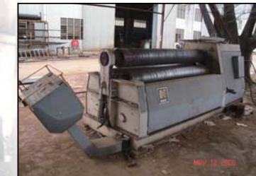
HACO 3HBR220 Rolling Machine Capacity : MS Plate Thickness 1mm ~ 12mm
