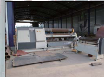
Haco Rolling Machine Capacity : MS Plate Thickness 1mm ~ 20mm
