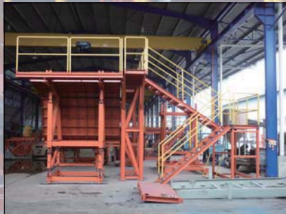
STEEL MOULD TRIAL ASSEMBLY
