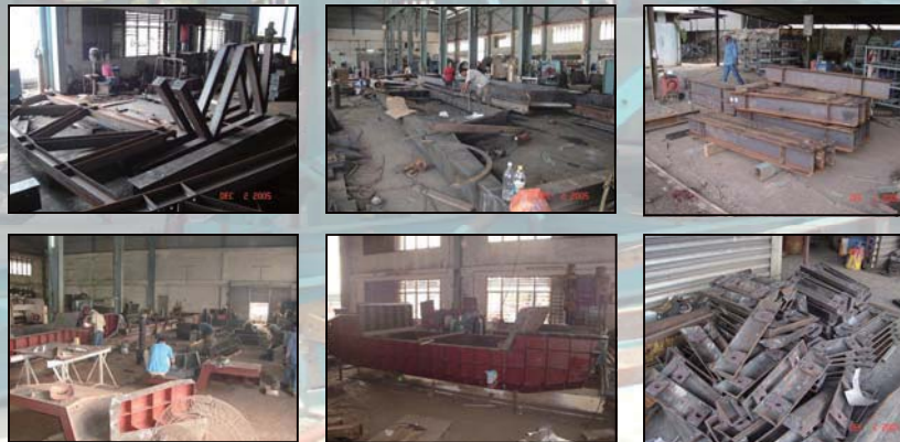
In-house fabrication Wing Form Support and Inner Core Form
