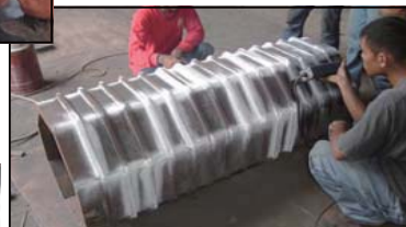
UT Test In Progress on Butt Weld.
