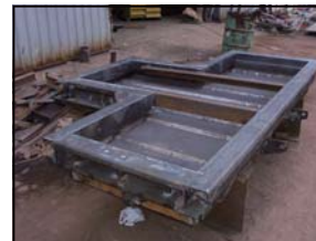
Parapet Steel Mould
