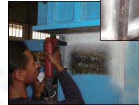
MPI Test on Pier Bracket & Internal Strut.
