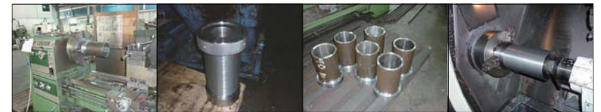
50 tons single acting jack machining in progress.
