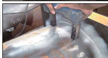
Magnetic Particle Inspection (MPI) Test In Progress on Fillet Weld.
